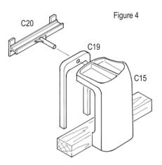
When soldering parts together, use a piece of strip wood to space cowl from chassis clip
