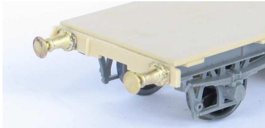
Because the flange at the base of each buffer projects above the headstocks, a small crescent shaped divot needs to be cut in each end at each buffer location with a 4mm chainsaw file. Each crescent should be about three boards wide and centred under the fourth board from each corner, but check the fit of the body against the underframe as work progresses.
