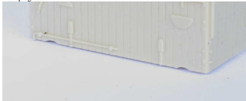
To attach the body to the underframe I followed the approach used by Graeme Brown on his four wheeled van, described in the August 2000 AMRM. Cement a piece of 1.5mm polystyrene sheet, 10mm x 30.5mm, inside each end of the body, spaced 0.8mm up from the base of the sides.
