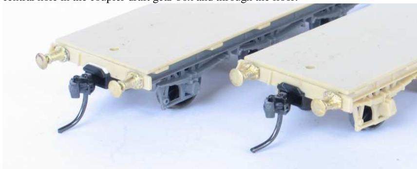
Now position the body on top of the underframe and use the 2.0mm drill to mark the position of the holes in the underside of the pieces of polystyrene glued in the body earlier. Drill 1.6mm holes on these marks and tap the holes M2. The body can be secured to the underframe with M2 x 8mm screws.
