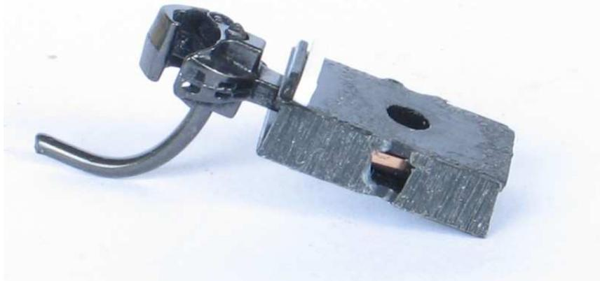
Cement the couplers to the underframe. Once the cement has hardened, use a 2.0mm drill to drill through the central hole in the coupler draft gear box and through the floor.
